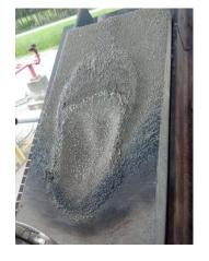
High Temperature Geopolymer panel tested at 4000°F at NASA Stennis.
