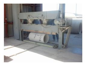
Geopolymer pipe about to be tested for D-load.
