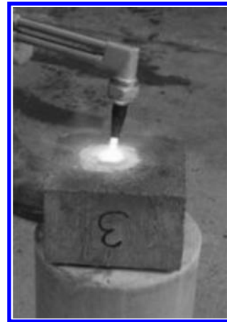
Figure 1. Geopolymer cube exposed to a flame of 1300°C.
