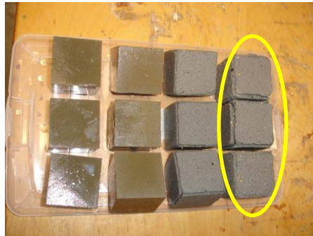
Class C fly ash Geopolymer
